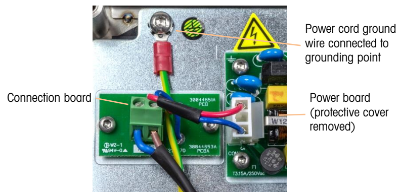
Figure 2-18: IND236 AC Power Connection Board and Grounding
