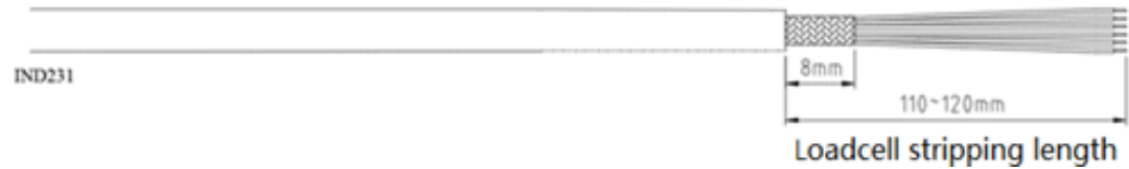
Figure 2-24: Load Cell Cable Stripping Length
