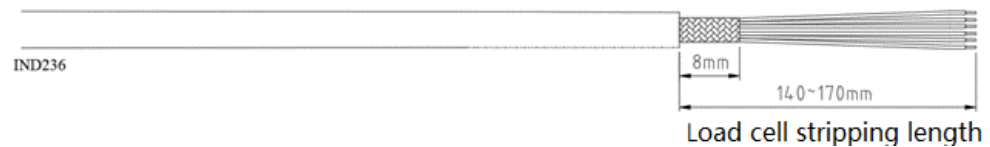
Figure 2-27: Load Cell Cable Stripping Length
